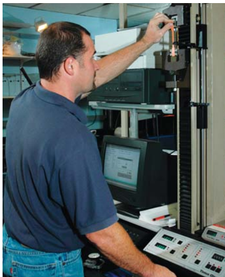
Bill Scott tests tensile strength of EPR compound.
